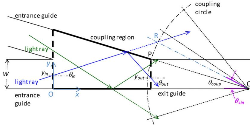
**Figure 3.** Asymmetric Y-coupler. The rays intersecting the coupling circle travel through the coupling region. Note that the propagation angle increases only when the ray reflects by the tilted surface such as the blue ray, while the propagation angle of the green ray does not change.
