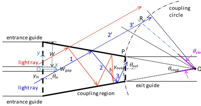
**Figure 2.** Symmetric Y-coupler. The blue ray travels through the coupling region and its extension intersects the coupling circle at R, located in the second mirror coupling region. The coordinate  $y_{out}$  and propagation angle  $\theta_{out}$  can be found using the coupling geometrics.
