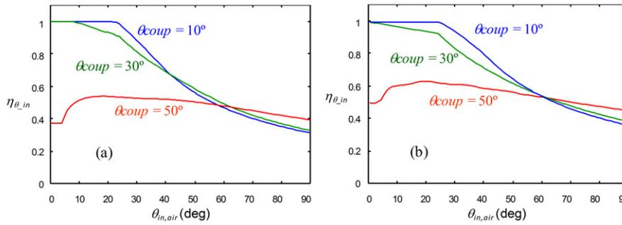
**Figure 5.** Accumulated coupling efficiency of symmetric and asymmetric Y-couplers with coupling angles of 10°, 30° and 50°.
