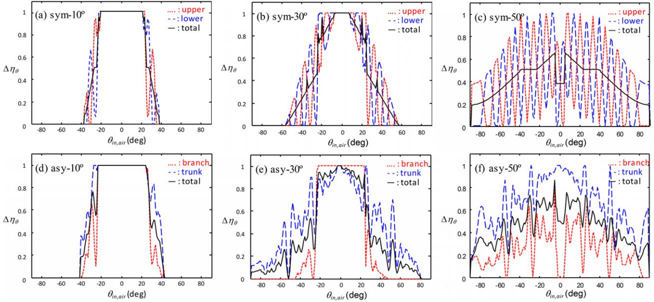
**Figure 4.** Angular coupling efficiency of symmetric and asymmetric Y-couplers with coupling angles of 10°, 30° and 50°. The efficiency profiles of the two entrance guides of the symmetric Y-coupler are similar, as shown in (a)–(c). For the asymmetric Y-couplers, the efficiency profiles of the trunk and the branch guides are considerably different, as shown in (d)–(f).
