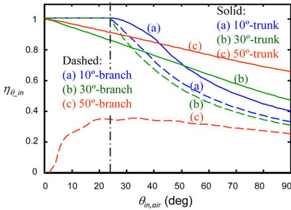
**Figure 6.** Accumulated coupling efficiency of individual light guides of asymmetric Y-couplers with coupling angles of 10°, 30° and 50°. The dash–dotted line indicates the incident angle (in air) to the light guide which can provide the highest coupling efficiency. It is 24° here and is used to specify the  $f/\#$  of the sunlight concentrator.
