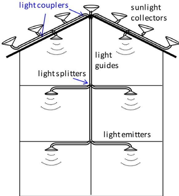
**Figure 1.** Schematic of a daylighting system with a building layout. Sunlight is gathered by the collectors and transferred to light emitters in a building through a light guiding system.
