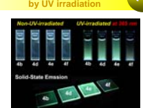
Fig. 6 Photographs of some polyamide solutions (10 -4 M) and thin films (thickness: 1–3 μm) by UV irradiation (excited at 365 nm).
