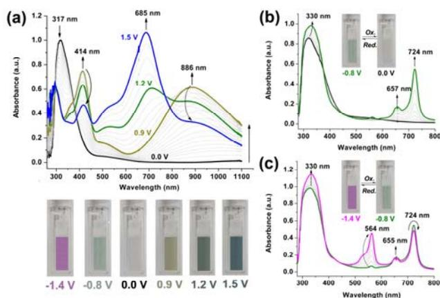
**Fig. 2** Spectral changes of the cast film of polyimide **3a** on the ITO-coated glass substrate on (a) p-doping in 0.1 M Bu<sub>4</sub>NClO<sub>4</sub>/CH<sub>3</sub>CN and (b, c) n-doping in 0.1 M Bu<sub>4</sub>NClO<sub>4</sub>/DMF at various applied potentials (vs. Ag/AgCl). The photographs show the color change of the film on an ITO electrode at indicated potentials.
