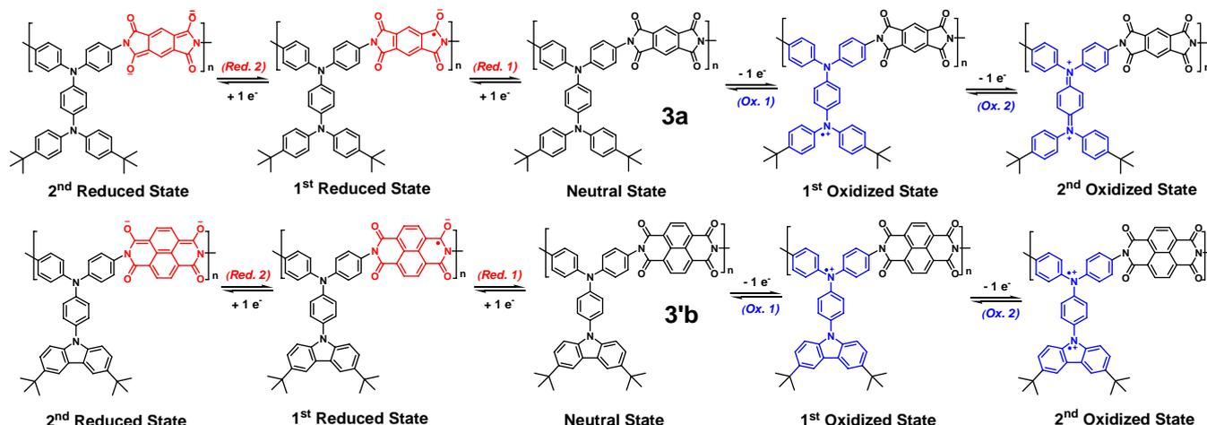
**Scheme 2.** Proposed redox chemistry of the polyimides **3a** and **3'b**
