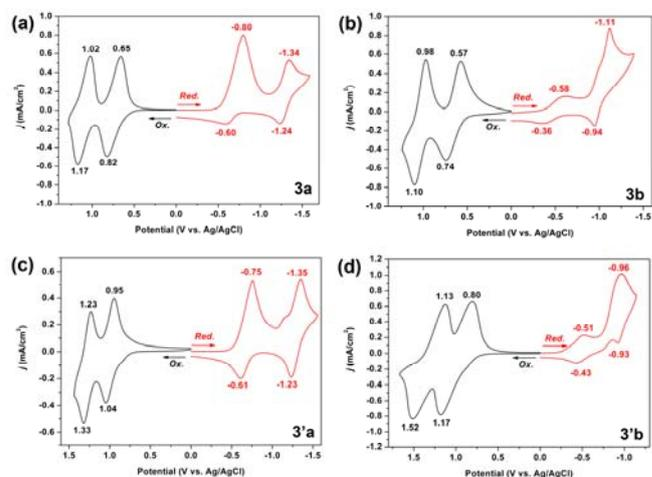
**Fig. 1.** Cyclic voltammetric diagrams of the cast films of polyimides (a) **3a**, (b) **3b**, (c) **3'a**, and (d) **3'b** on an ITO-coated glass substrate in 0.1 M  $\text{Bu}_4\text{NClO}_4/\text{acetonitrile}$  (for p type doping) and DMF (for n type doping) solution at a scan rate of 50 mV/s, respectively.
