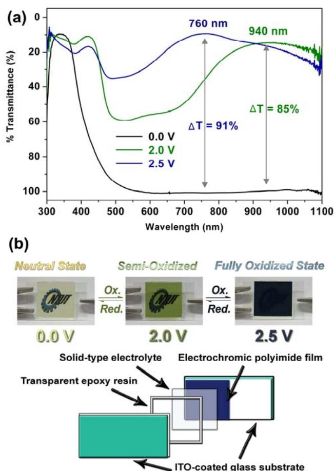
**Fig. 4** (a) Transmittance spectra of single-layer ITO-coated glass ECD, using polyimide **3a** as active layer. (b) Photographs and schematic diagram of polyimide EDC.
