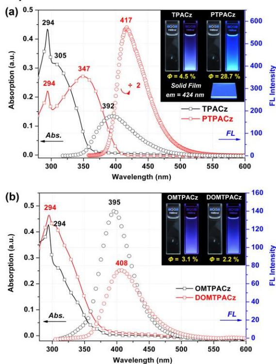
**Figure 4.** UV-Vis absorption and PL spectra of the dilute solutions of (a) TPACz and PTPACz (b) MeOTPACz and (MeOTPACz)<sub>2</sub> in  $\text{CH}_2\text{Cl}_2$  ( $1 \times 10^{-5}$  M). Quinine sulfate dissolved in 1 M  $\text{H}_2\text{SO}_4$  (aq.) with a concentration of  $1 \times 10^{-5}$  M as the standard ( $\Phi_F = 54.6\%$ ). Photos show PL images of the solutions upon UV exposure (excited at 365 nm).
