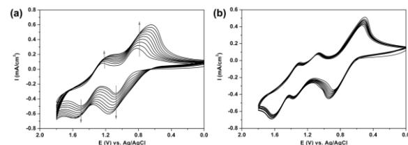
**Figure 3.** Repeated potential scan of (a) TPACz and (b) MeOTPACz monomers scan at rate 150 mV/s between 0 and 1.8 V in 0.1 M  $\text{Bu}_4\text{NClO}_4/\text{MeCN}$  solution.
