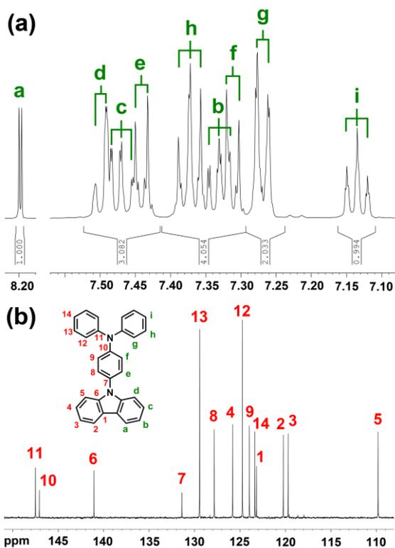
**Figure 1.** (a)  $^1\text{H}$  NMR and (b)  $^{13}\text{C}$  NMR spectra of TPACz in  $\text{CDCl}_3$ .
