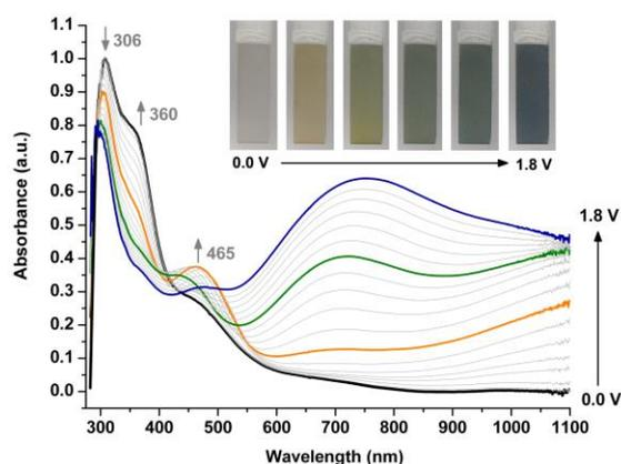
**Figure 8.** Spectroelectrochemical spectra of **PTPACz** with applied potential between 0 and 1.8 V in  $\text{Bu}_4\text{NClO}_4/\text{CH}_3\text{CN}$  solution.
