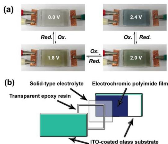
**Figure 9.** (a) Photos of sandwich-type ITO-coated plastic single layer electrochromic device, using **PTPACz** as active layer. (b) Schematic illustration of the structure of the ECD.
