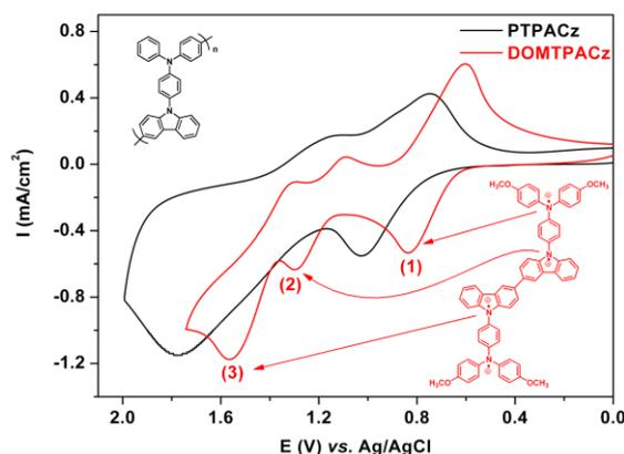
**Figure 7.** Cyclic voltammogram of **PTPACz** and the **(MeOTPACz)<sub>2</sub>** dimer in 0.1 M  $\text{Bu}_4\text{NClO}_4/\text{CH}_3\text{CN}$  solution at scan rate 50 mV/s.
