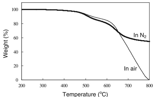
**Fig. 12** TGA curves of the poly(ester-imide) *m-8c* in nitrogen and air (heating rates of 20 °C/min)
