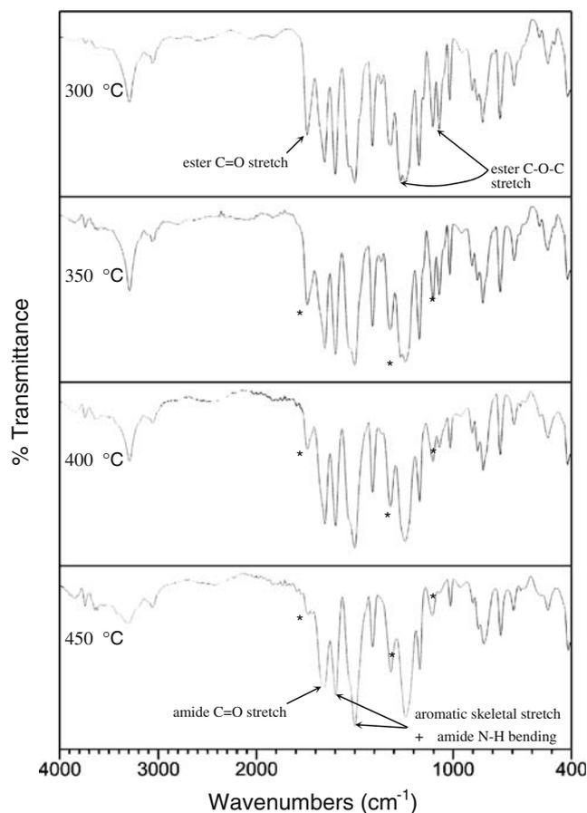
**Fig. 10** FT-IR spectra (thin-film sample) of the poly(ester-amide) *p-5h* after sequential heating in air at the indicated temperatures, each for 10 min (asterisk indicates the characteristic absorptions of the ester groups)
