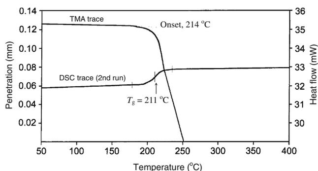
**Fig. 8** Typical DSC and TMA thermograms of the poly(ester-amide) *p-5i*: DSC, heating rate of 20 °C/min; TMA, heating rate of 10 °C/min and applied force of 10 mN
