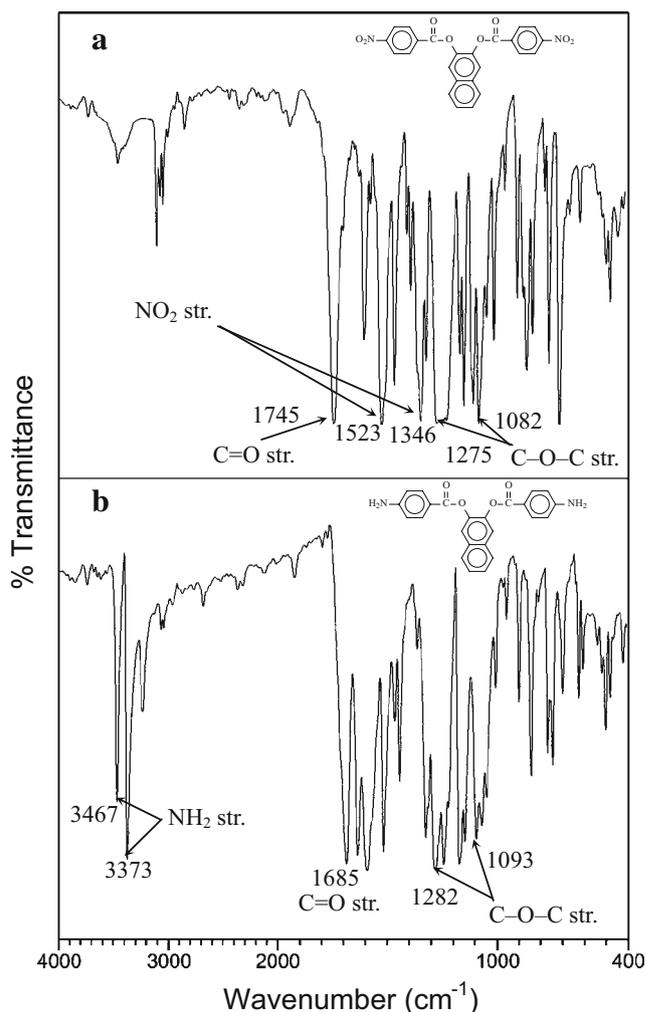
**Fig. 1** FT-IR spectra of **a** the dinitro-diester *p*-1 and **b** the bis(ester-amine) *p*-2
