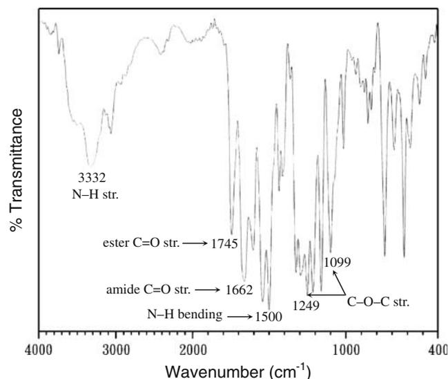
**Fig. 5** FT-IR spectrum of a thin film of the copoly(ester-amide) *m-5j*
