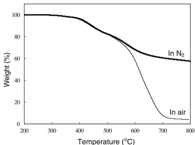
**Fig. 9** TGA curves of the poly(ester-amide) *p-5j* in nitrogen and air (heating rates of 20 °C/min)
