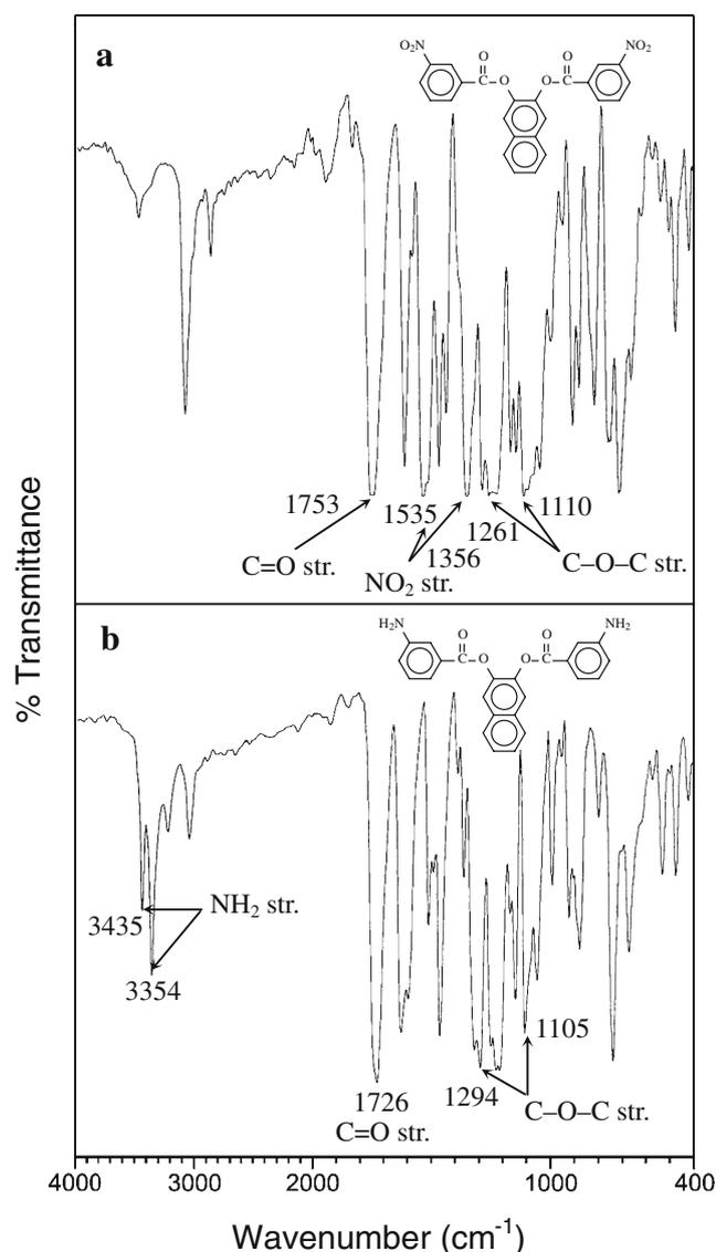
**Fig. 2** FT-IR spectra of **a** the dinitro-diester *m-1* and **b** the bis(ester-amine) *m-2*
