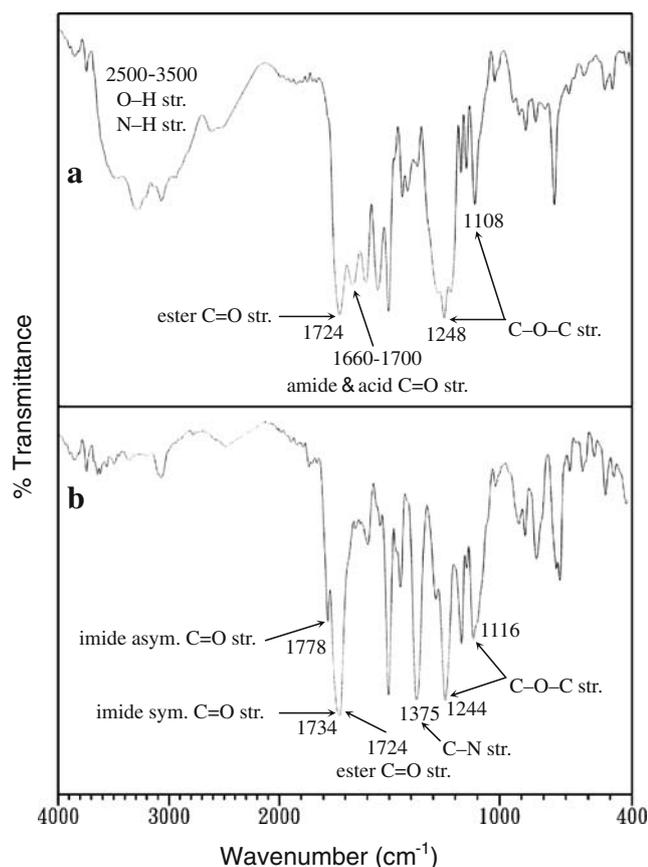
**Fig. 6** FT-IR spectra of **a** the poly(amic acid) precursor *m-7d* and **b** the poly(ester-imide) *m-8d*
