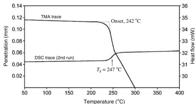
**Fig. 11** Typical DSC and TMA thermograms of the poly(ester-imide) *m-8d*: DSC, heating rate of 20 °C/min; TMA, heating rate of 10 °C/min and applied force of 10 mN
