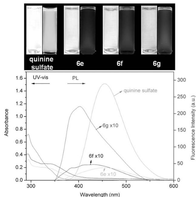
**Fig. 7** UV-vis and PL spectra of solutions of poly(amine-imide)s **6e**, **6f**, and **6g** in NMP ( $1 \times 10^{-5}$  M). A solution of quinine sulfate in 1 N  $\text{H}_2\text{SO}_4$  (aq) with a concentration of  $1 \times 10^{-5}$  M was used as the reference standard ( $\Phi_F = 0.546$ ). Photographs show the appearance of the sample solutions before and after exposure to a standard laboratory UV lamp.
