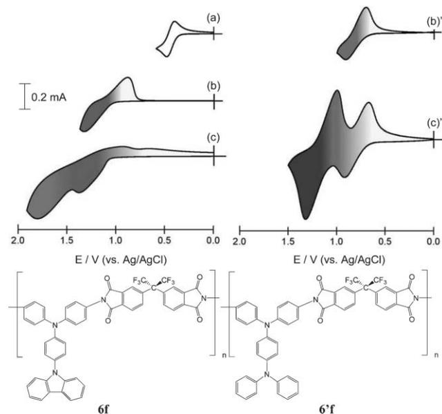
**Fig. 9** Cyclic voltammograms of the cast films of poly(amine-imide) **6f** and **6'f** on an ITO-coated glass substrate in 0.1 M TBAP- $\text{CH}_3\text{CN}$  at a scan rate of  $100 \text{ mV s}^{-1}$ . (a) Ferrocene; (b), (b') first redox couple; (c), (c') first and second redox couples.
