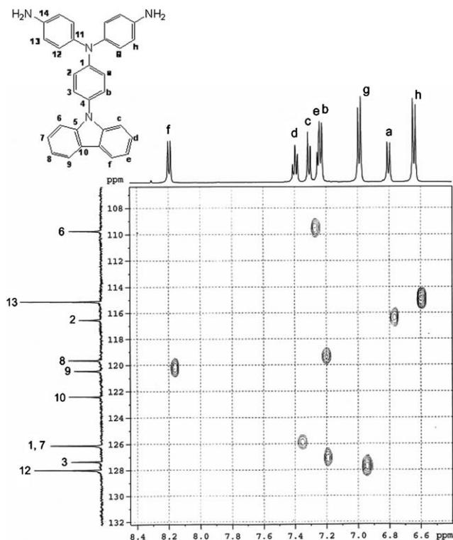
Fig. 3 C-H COSY spectrum of diamine 4 in  $\text{DMSO}-d_6$ .
