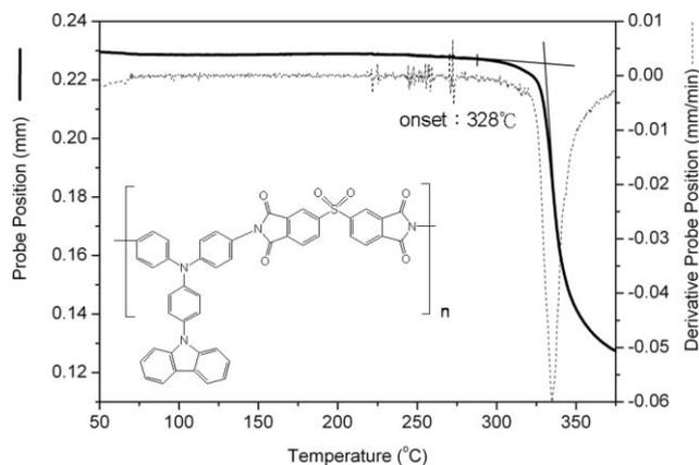
**Fig. 6** TMA curve of poly(amine-imide) **6e** with a heating rate of 10 °C min<sup>-1</sup>.
