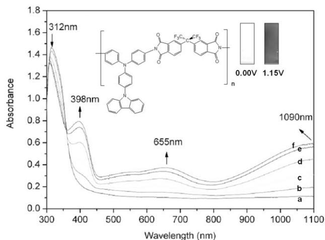
**Fig. 10** *In situ* spectroelectrochemical series of a cast film of poly(amine-imide) **6f** in 0.1 M TBAP-CH<sub>3</sub>CN at various applied potentials vs. Ag/Ag<sup>+</sup>: (a) 0.00, (b) 0.90, (c) 1.00, (d) 1.05, (e) 1.10, and (f) 1.15 V.
