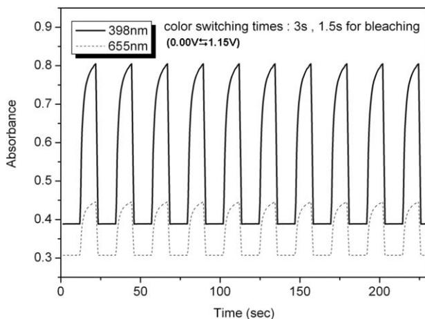
**Fig. 11** Variation of absorbance for a cast film of poly(amine-imide) **6f** as a function of time for ten switches between 0.00 and 1.15 V vs. Ag/Ag<sup>+</sup> in 0.1 M TBAP-CH<sub>3</sub>CN.
