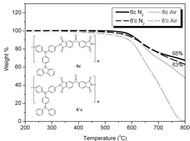
**Fig. 5** TGA thermograms of poly(amine-imide) **6c** and **6'c** at a scan rate of 20 °C min<sup>-1</sup>.
