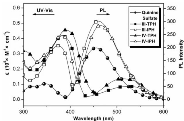
**Figure 7.** UV-vis absorptions and PL spectra of poly(amine-1,3,4-oxadiazole)s in NMP solution ( $10^{-5}$  M). Quinine sulfate dissolved in 1 N  $\text{H}_2\text{SO}_4(\text{aq})$  ( $10^{-5}$  M) as the standard. ( $\Phi_F = 0.546$ .)
