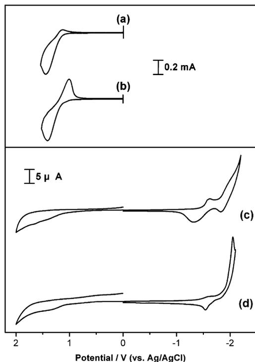
**Figure 10.** Cyclic voltammograms of poly(amine-hydrazide) (a) **I-TPH** and (b) **II-TPH** and poly(amine-1,3,4-oxadiazole) (c) **III-TPH** and (d) **IV-TPH** films onto an indium-tin oxide (ITO) coated glass substrate in  $\text{CH}_3\text{CN}$  (oxidation) and DMF (reduction) solution containing 0.1 M TBAP at scan rate = 0.1 V/s.
