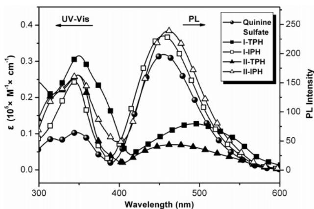
**Figure 6.** UV-vis absorptions and PL spectra of poly(amine-hydrazide)s in NMP solution ( $10^{-5}$  M). Quinine sulfate dissolved in 1 N  $\text{H}_2\text{SO}_4(\text{aq})$  ( $10^{-5}$  M) as the standard. ( $\Phi_F = 0.546$ .)
