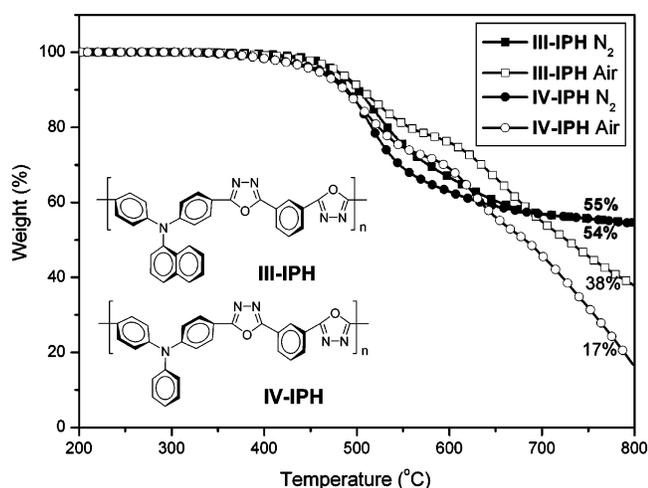
**Figure 5.** TGA thermograms of poly(amine-1,3,4-oxadiazole)s **III-IPH** and **III-IPH** at a scan rate of 20 °C/min.
