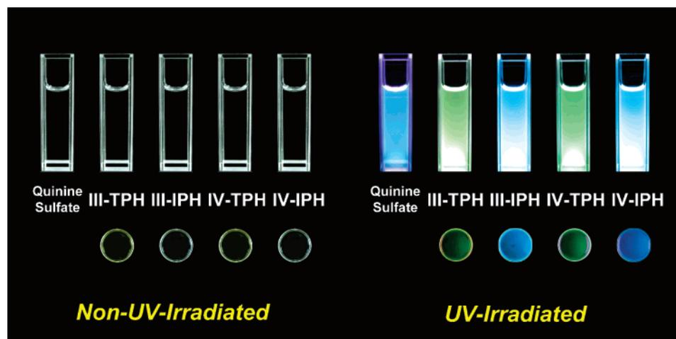
**Figure 9.** Photoluminescence of poly(amine-1,3,4-oxadiazole) solutions ( $10^{-5}$  M) and thin films (thickness:  $1-3 \mu\text{m}$ ) by UV irradiation (Excited at 365 nm). Quinine sulfate dissolved in 1 N  $\text{H}_2\text{SO}_4(\text{aq})$  ( $10^{-5}$  M) as the standard. ( $\Phi_F = 0.546$ .)
