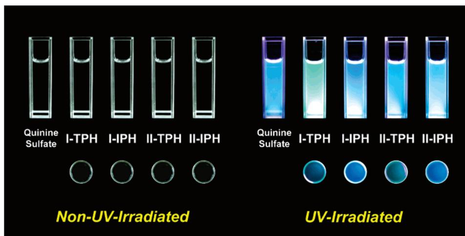
Figure 8. Photoluminescence of poly(amine–hydrazide) solutions ( $10^{-5}$  M) and thin films (thickness:  $1\text{--}3\ \mu\text{m}$ ) by UV irradiation (excited at 365 nm). Quinine sulfate dissolved in 1 N  $\text{H}_2\text{SO}_4(\text{aq})$  ( $10^{-5}$  M) as the standard. ( $\Phi_F = 0.546$ .)
