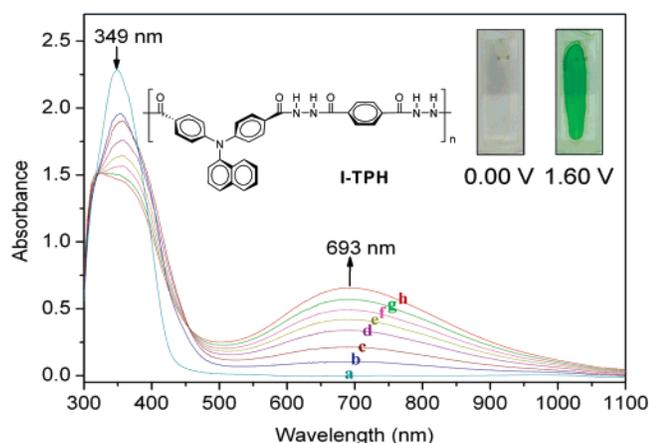
**Figure 12.** Electrochromic behavior of poly(amine-hydrazide) **I-TPH** thin film (in  $\text{CH}_3\text{CN}(\text{aq})$  with 0.1 M TBAP as the supporting electrode) at (a) 0.00, (b) 1.00, (c) 1.10, (d) 1.20, (e) 1.30, (f) 1.40, (g) 1.50, (h) and 1.60 V.
