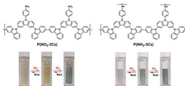
Fig.1: Structures and electrochromism of the electrodeposited polycarbazole films.
