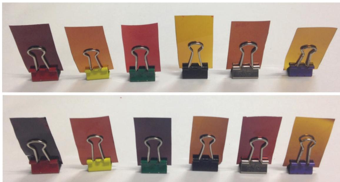
**Figure 5.** Photographs of the thermally cured films of polyimides **5a** → **5f** (top) and **6a** → **6f** (bottom) with film thickness of about 70  $\mu\text{m}$ .
