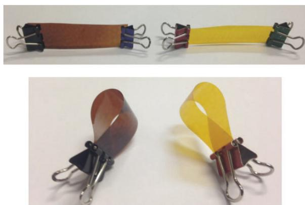
**Figure 6.** Photographs of the thermally (left) and chemically (right) imidized films of polyimide **5f**.
