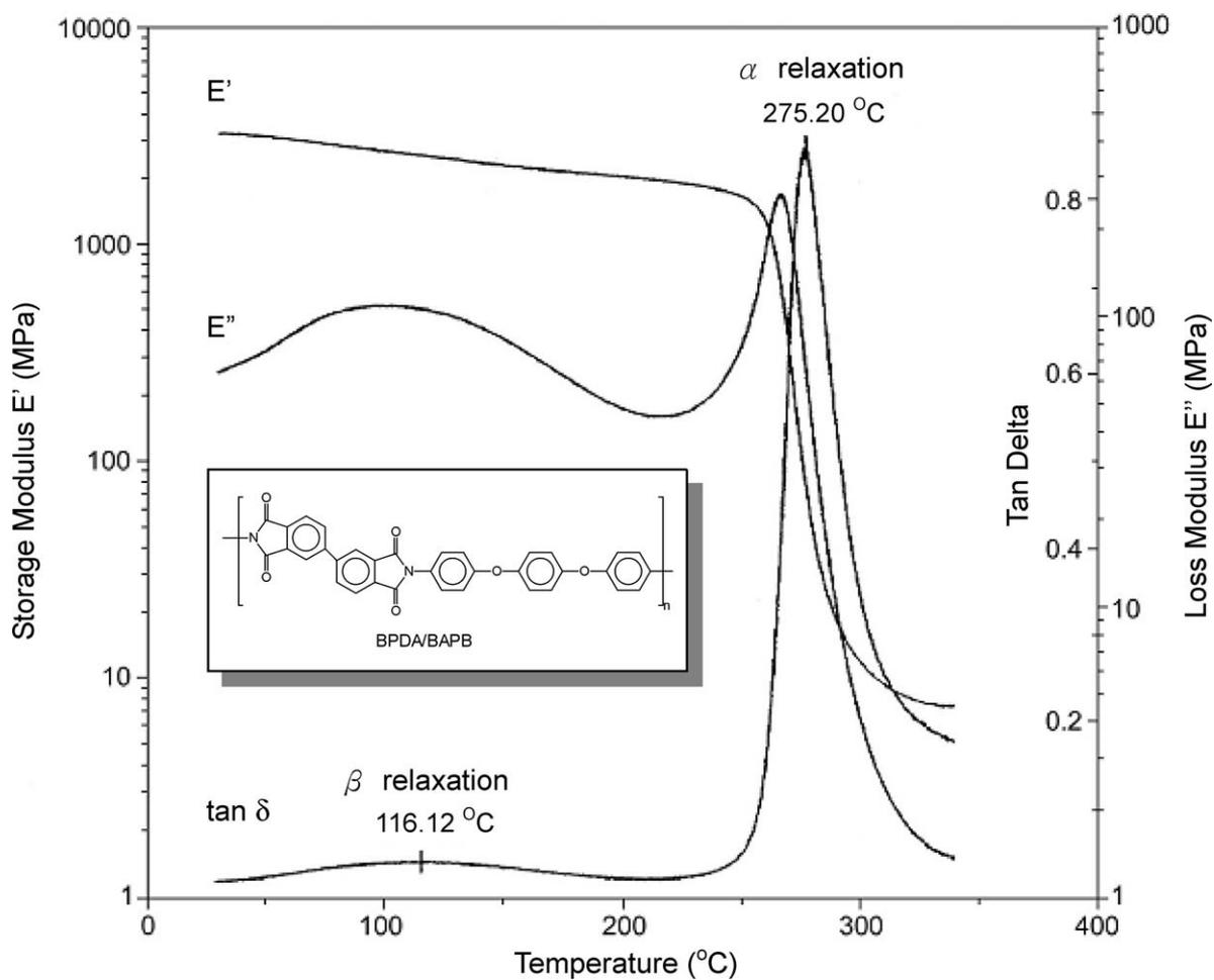
Figure 7. DMA curves of the BPDA/BAPB polyimide. Sample size = 14 × 5 × 0.07 mm; Amplitude = 30 μm; Autotension = 125%; Frequency = 1 Hz; Scan rate = 5 °C/min.
