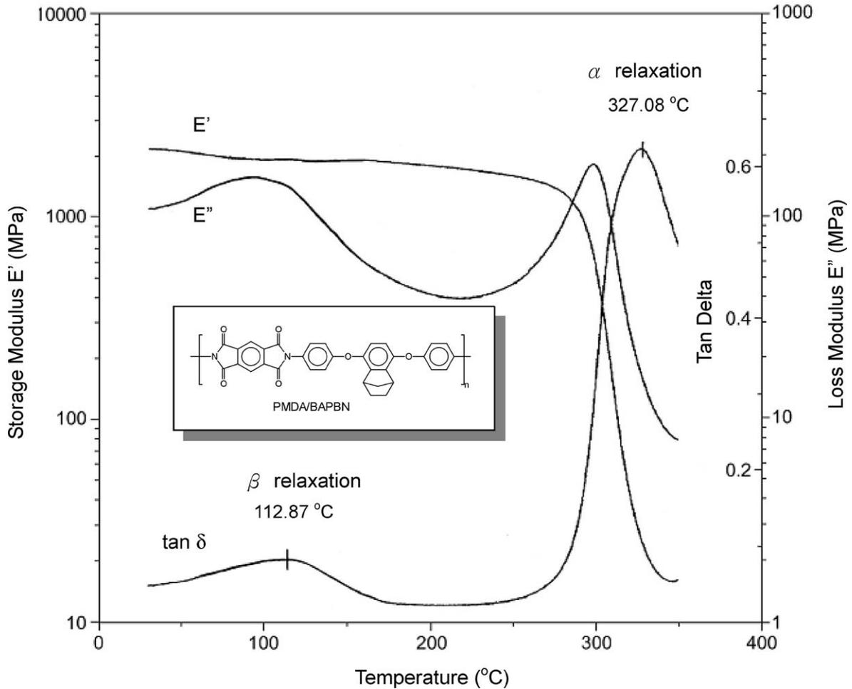
Figure 6. DMA curves of the PMDA/BAPBN polyimide. Sample size = 14 × 5 × 0.08 mm; Amplitude = 30 μm; Autotension = 125%; Frequency = 1 Hz; Scan rate = 5 °C/min.
