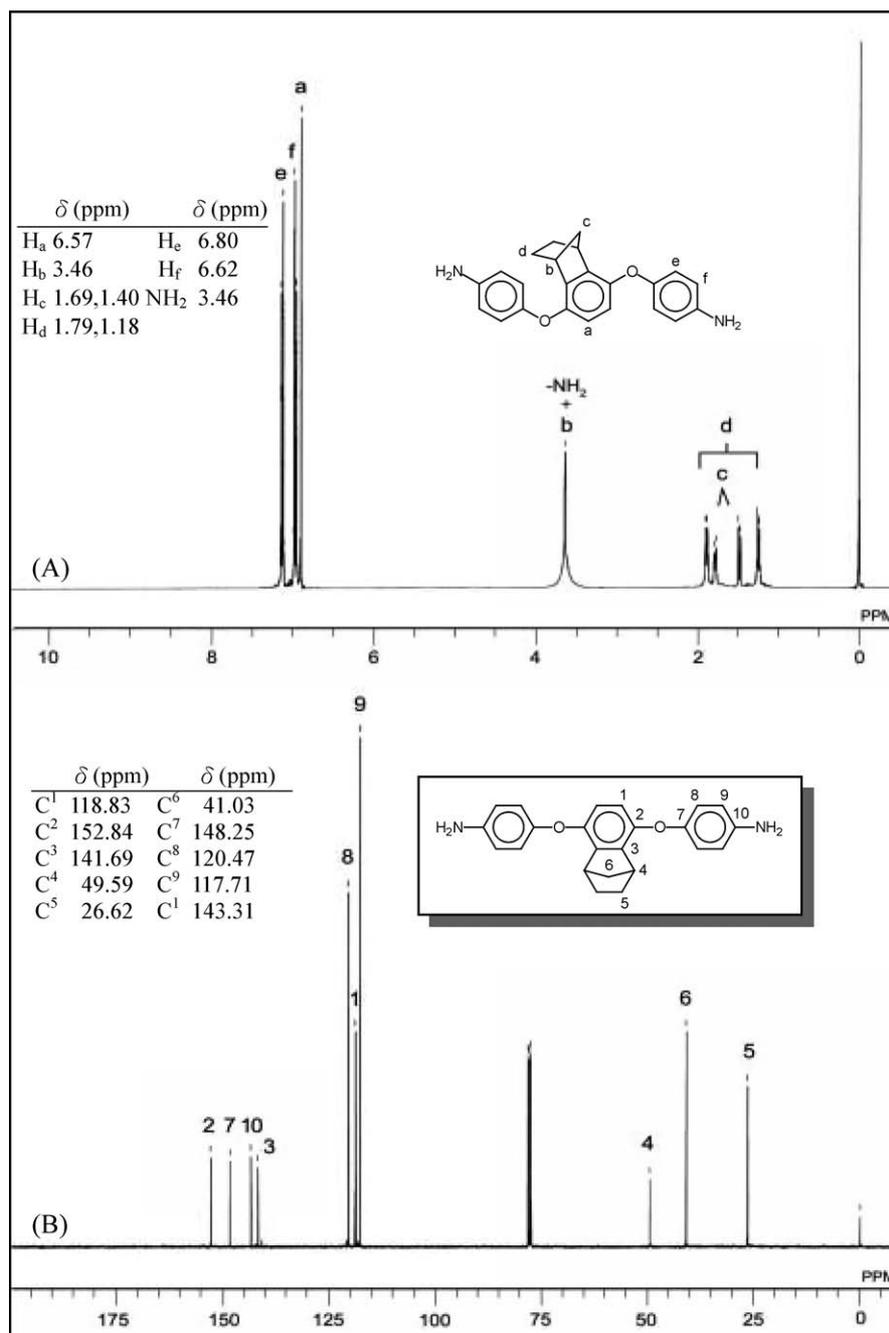
Figure 2.  $^1\text{H}$  NMR (A) and  $^{13}\text{C}$  NMR (B) spectra of diamine BAPBN in  $\text{CDCl}_3$ .
