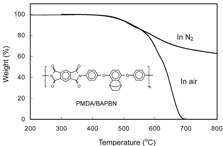
Figure 8. TGA curves of PMDA/BAPBN polyimide (Heating rate = 20 °C/min).
