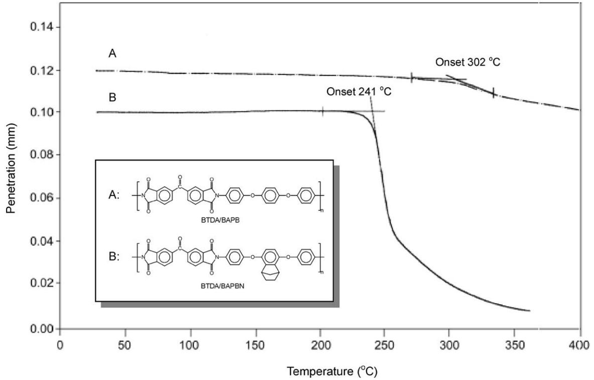
Figure 5. TMA thermograms of polyimides BTDA/BAPB and BTDA/BAPBN. Heating rate = 10 °C/min; DC force = 10 mN.
