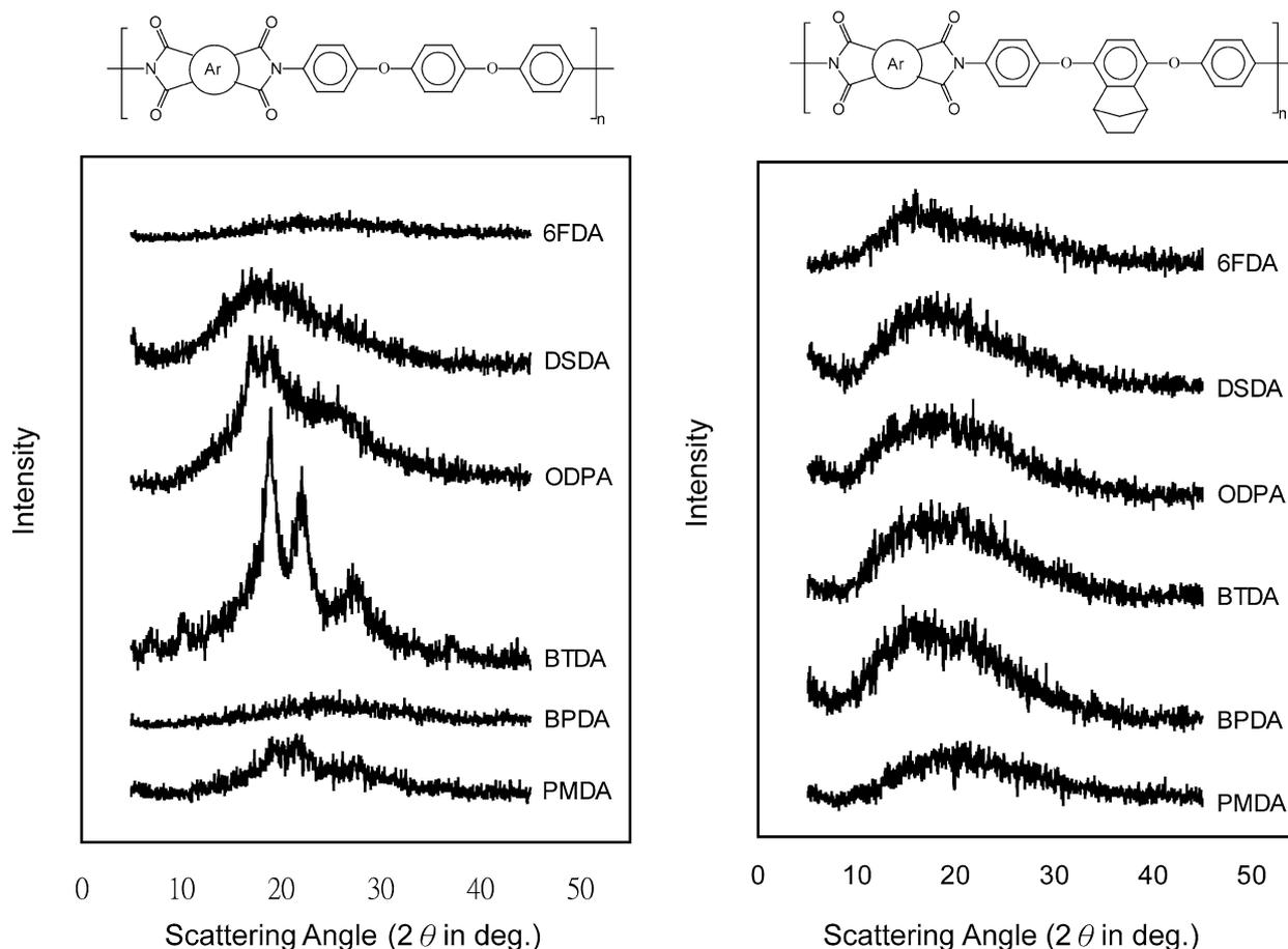
Figure 4. X-ray diffraction patterns of some BAPB and BAPBN polyimides.
