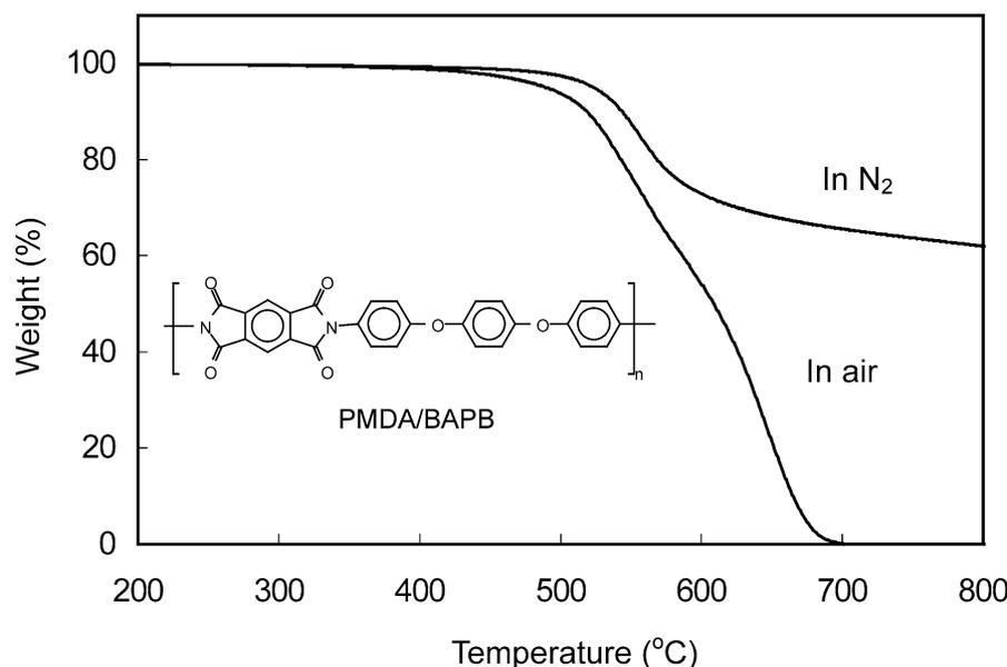
Figure 9. TGA curves of PMDA/BAPB polyimide (Heating rate = 20 °C/min).
