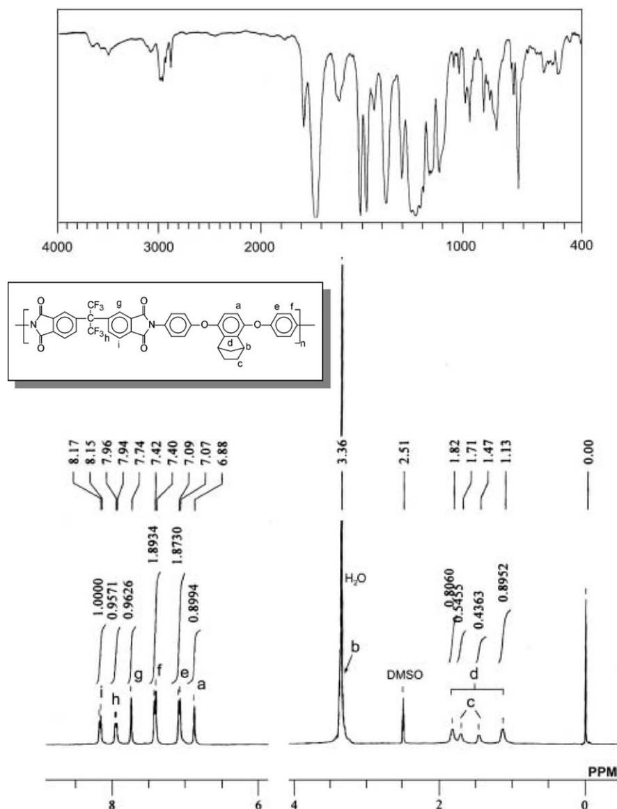
Figure 3. The typical set of IR and <sup>1</sup>H NMR (in DMSO-*d*<sub>6</sub>) spectra of 6FDA/BAPBN polyimide.
