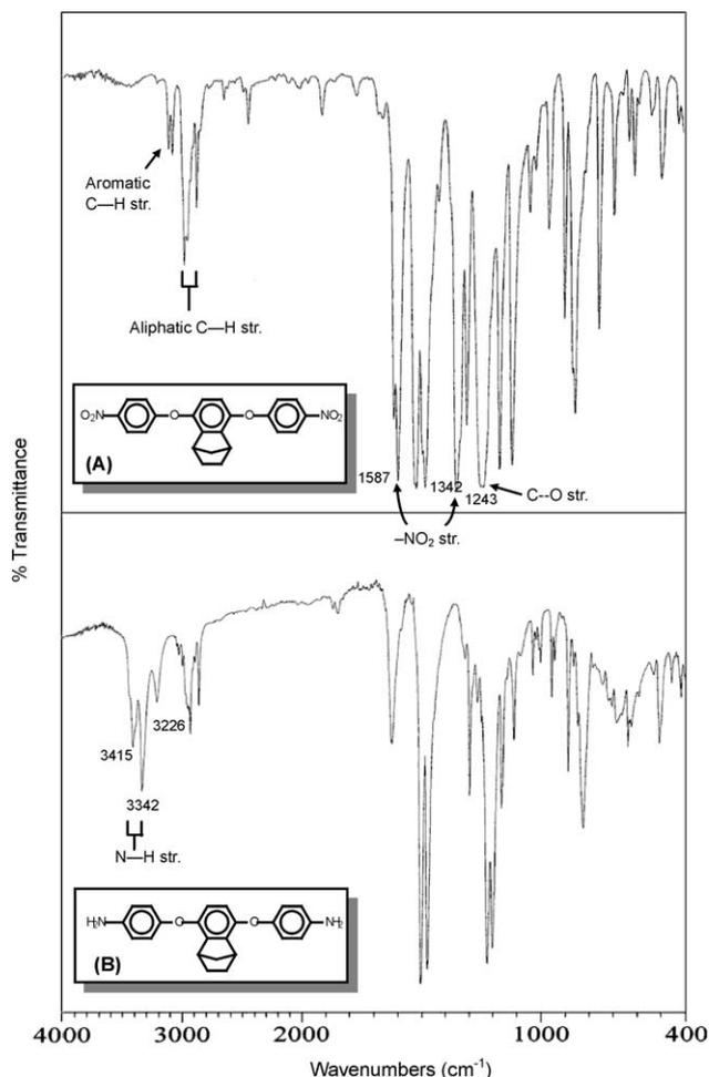
Figure 1. IR spectra of (A) dinitro compound BNPBN and (B) diamine BAPBN.
